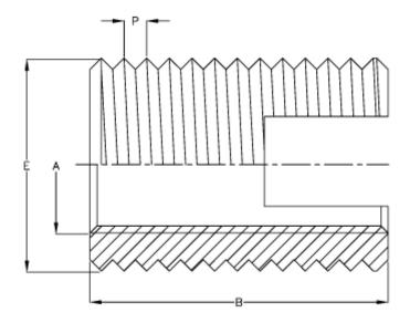
Female thread A = M2,5Length B = 6Male thread E = 4.5Min hole depth blind hole = 8
